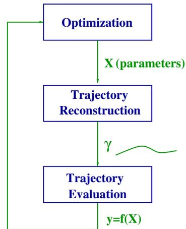
**Fig. 1** .The optimization process control the  $X$  vector in order to build a trajectory  $\gamma$  for evaluation.
