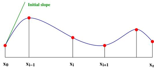
**Fig. 7** Piecewise cubic interpolation. The derivative at point  $x_i$  is given by line joining the point  $(x_{i-1}, y_{i-1})$  and  $(x_{i+1}, y_{i+1})$ . Between two points, a cubic polynomial is fitted. The term  $h$  represents the distance two consecutive points.
