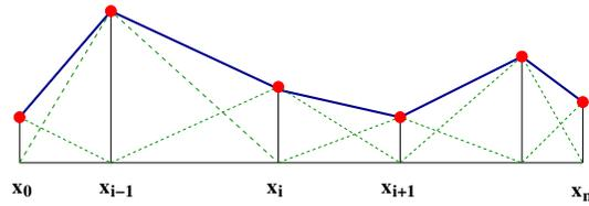
**Fig. 5** Piecewise linear interpolation.
