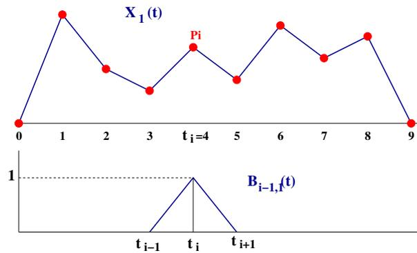
Fig. 12 Uniform B-Splines of Degree One
