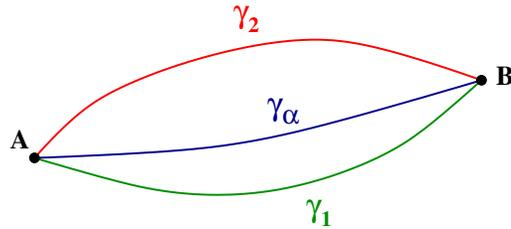
**Fig. 15** One new trajectory is built by using a weighted sum of two reference trajectories.
