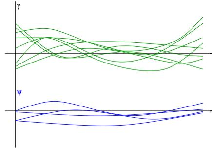
In the example presented in figure 14 a set of trajectories  $\gamma_i(t), i = 1 \dots n$  are used to build  $K = 4$  principal components ( $\psi_k(t)$ ) which can be used to reconstruct the initial trajectories.
