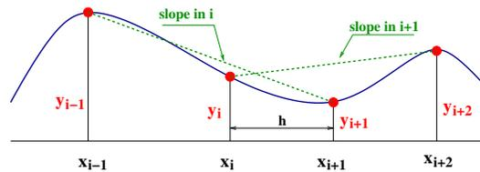
Moving a point do not affect all the curve which is the main advantage of this interpolation. The resulting curve is  $C^1$  but not  $C^2$  (the second derivative is not continuous). The curvature radius of a curve may be expressed by the following expression :
