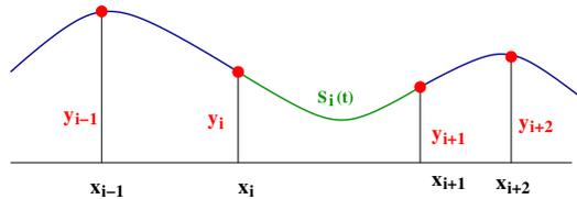
**Fig. 8** Cubic Spline Interpolation.
