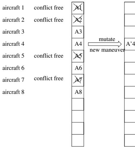
Fig. 5. Adapted mutation operator.
