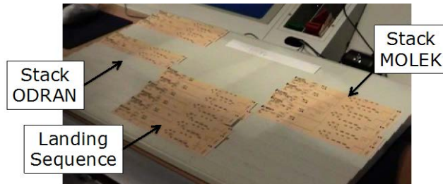
Fig. 2. The flight strips on the strip board are organized into three groups. The upper left and right groups contain the strips for aircraft in each of the two stacks. The centre group holds the strips for the aircraft that have left the stack and are approaching the runway beacon.
