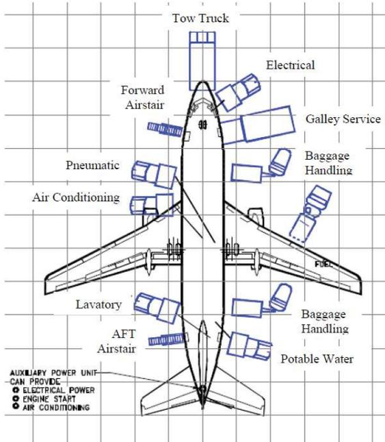
Figure 2: Ground handling arrangement [2] .
