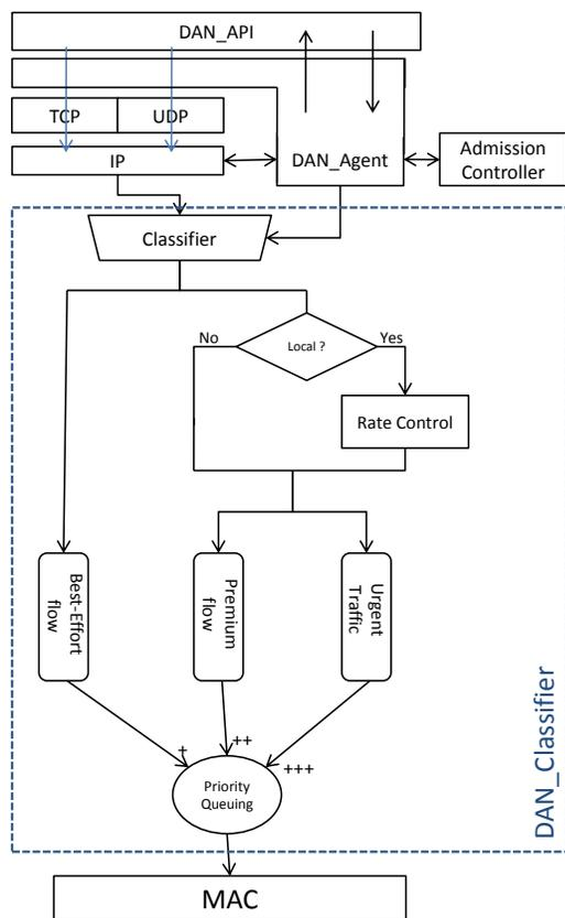
Fig. 2. DAN Mechanisms
