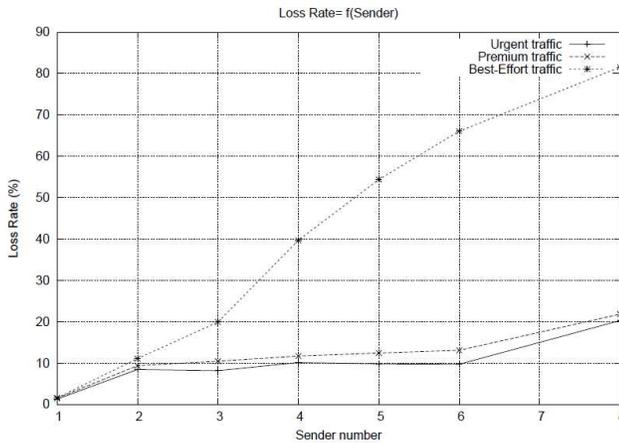
Fig. 4. Average Loss Rate vs. number of Senders
