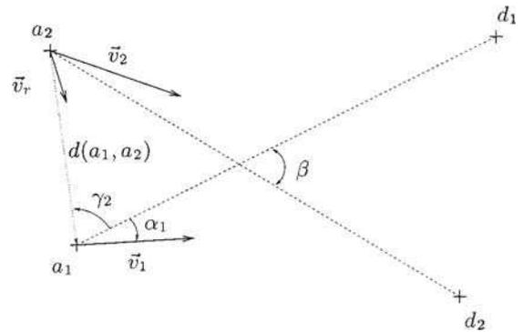
Figure 1. The neural network inputs of aircraft 1.
