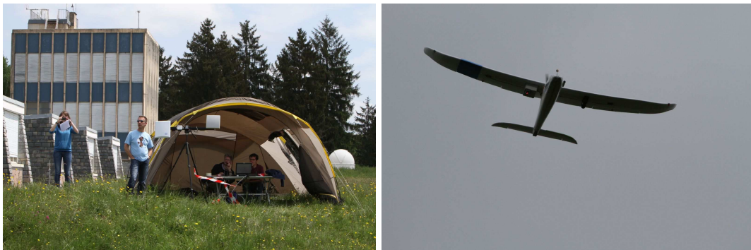
Figure 6: Third campaign at Lannemezan. Left: base camp. Right: EasyStar equipped with a cloud sensor (right wing), a video recorder (left wing) and a static electricity sensor (noise).
