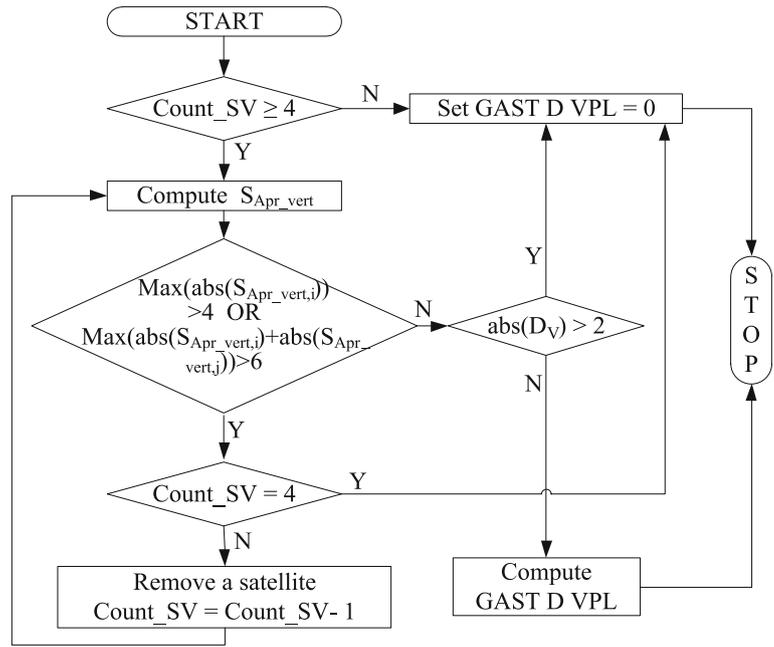
Step 2. GAST D VPL is equal to 0 indicates that the GBAS system could not meet the requirements of Approach Service Type D at that epoch
