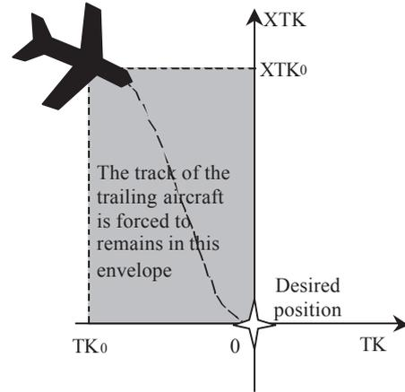
Figure 3 Track envelope of the trailing aircraft
