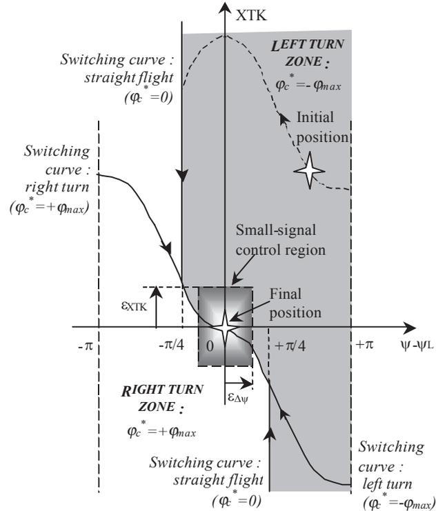
Figure 5 Modified 'cross track' suboptimal control law
