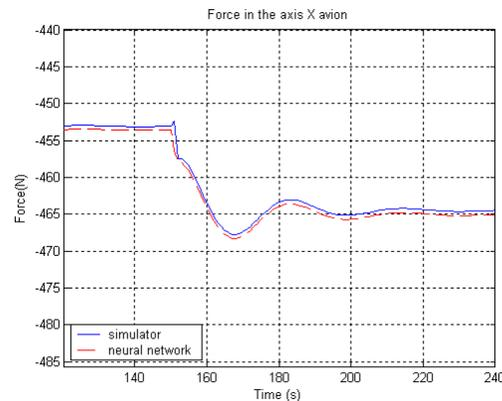
**Figure 5. Estimated and computed longitudinal force  $F_x$**
