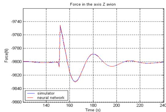
**Figure 6. Estimated and computed longitudinal force  $F_z$**
