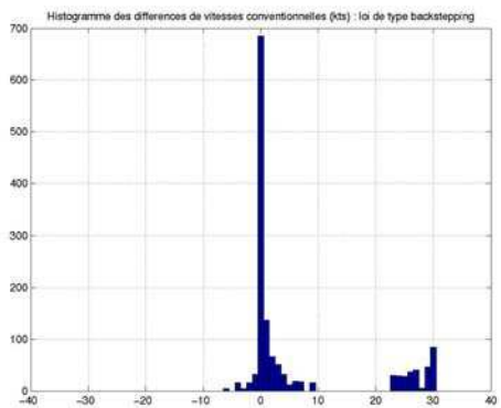
Figure 13. Difference between the conventional airspeed of the two aircraft at the sequencing measurement point with the nonlinear feedback loop
