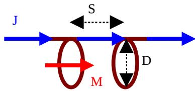
**Figure 4: Co-located magnetic (M) and electric (J) dipoles**
