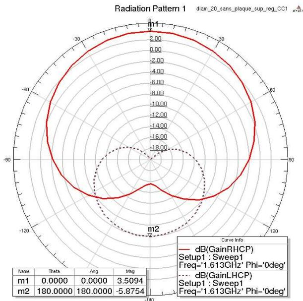
Figure 7: Antenna RHCP and LHCP gain pattern (dBi)
