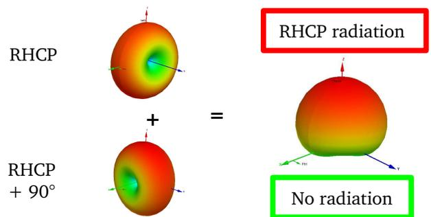
Figure 3: Half-directional radiation pattern
