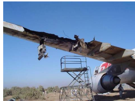
Fig. 1 The damaged left wing after landing
