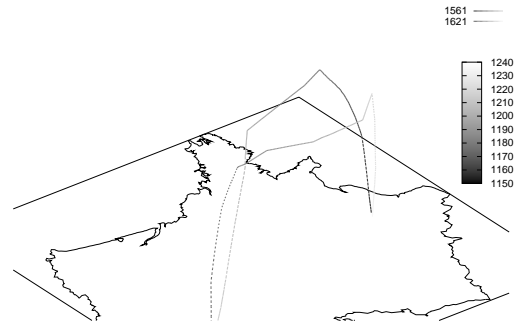
Figure 2. Three potential conflicts between two flights: one near Paris airport at low altitude and two other en-route at the cruising altitude of the lower flight. The gray scale corresponds to time (in minutes) along the trajectory, the lighter the later.
