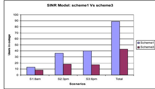
**Figure 5. Reuse scheme 1 and scheme 3 results with 3 scenarios**
