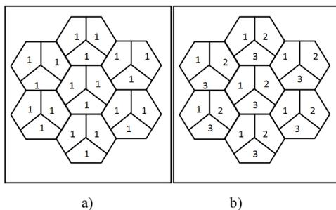
Figure 1. Seven-cell hexagonal layout. a) 1x3x1 b) 1x3x3
