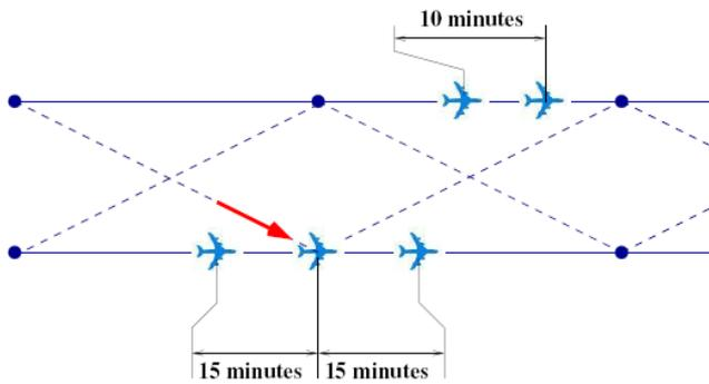
Figure 2. Aircraft longitudinal separation criterion on the tracks
