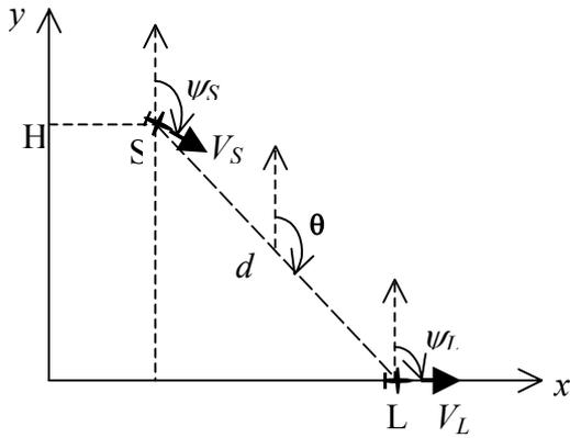
Figure 2 : Relative position of aircraft
