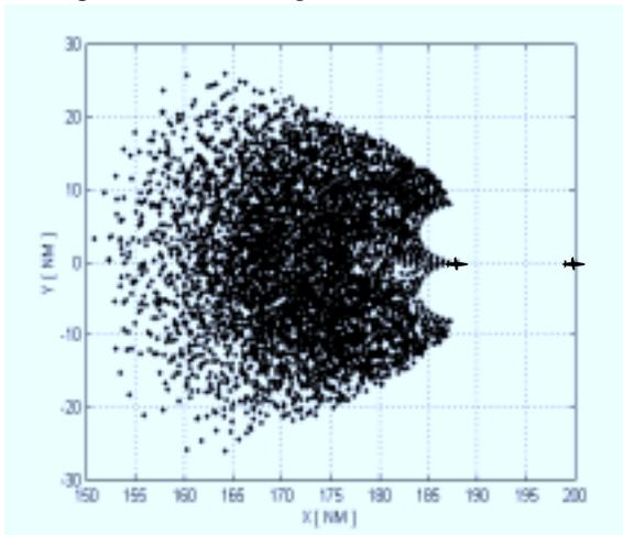
**Figure 6:** Discretization of the convergence maneuver relative space.
