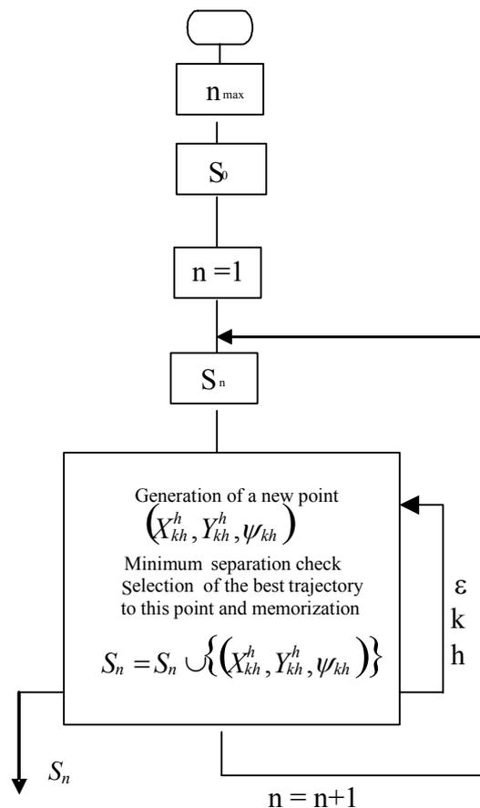
**Figure 5:** Inverse generation of optimal convergence trajectories sets.
