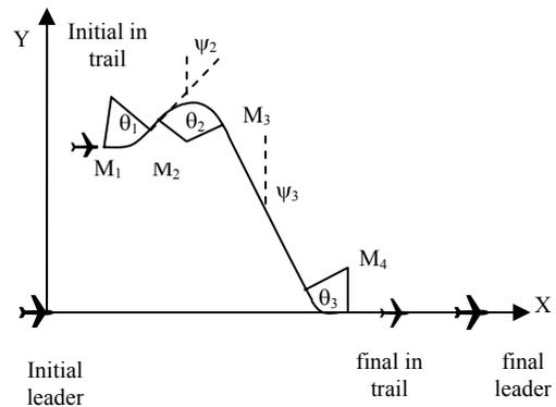
**Figure 4 :** Representation of a regular convergence trajectory.
