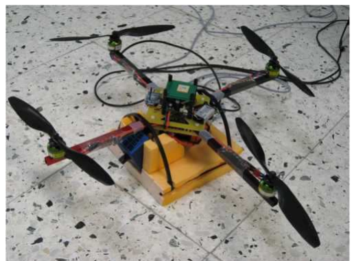
Fig. 1: The ENAC micro-UAV with the SwissRanger SR-3000 and the IMU XSens MTi
