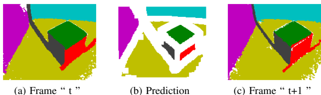
Fig. 9: Planes Tracking and Matching across a sequence of frames. By eroding frame “ t ”, planes are predicted in frame “ t+1 ”
