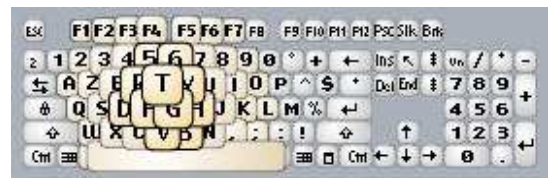
Figure 1: animation applied on fisheye keyboard when the stylus is closest to the key 'T'
