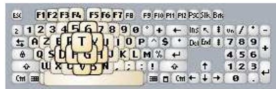
Figure 1: animation applied on fisheye keyboard when the stylus is closest to the key 'T'
