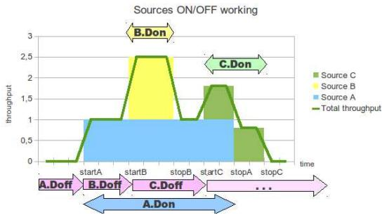
**Figure 1: Emission process of ON/OFF traffic sources**
