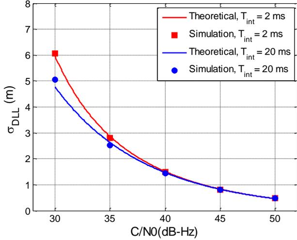
Fig. 2. DLL tracking error due to thermal noise
