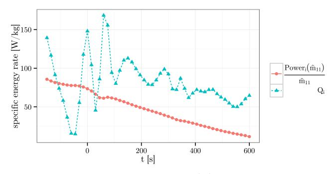
Figure 1: This figure portrays the computed specific energy rate  $\frac{Power_i(\hat{m}_{11})}{\hat{m}_{11}}$  and the observed specific energy rate  $Q_i$ . In this figure,  $\hat{m}_{11}$  was estimated with the least squares method. The largest error on the predicted altitude at the time t = 600s is obtained with this trajectory.
