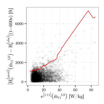
$e^{[1:11]}(\hat{m}_{11}^{LS})$ Figure 3: Relation between and absolute the predicted altitude the error on  $\left| H_p^{(pred)}(\hat{m}_{11}^{LS}) - H_p^{(obs)} \right| (t = 600 \text{ s}).$ The red line is the estimated 95 % quantile. It is obtained by local linear quantile regression [28].
