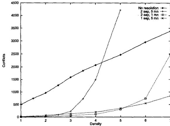
Figure 3: Number of separation losses vs density
