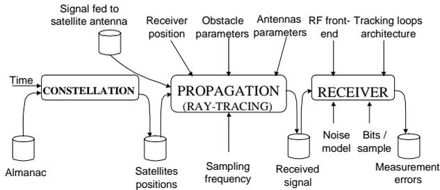
Figure 1: Architecture of the end-to-end GPS simulator.
