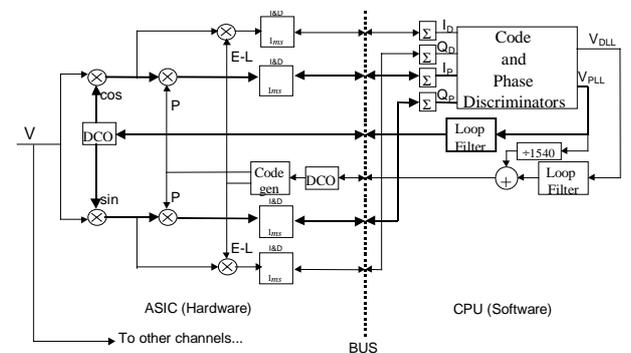
Figure 4: Architecture of a digital GPS receiver.
