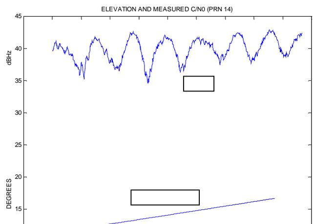
Figure 5: Measured  $C/N_0$  for a choke ring antenna 6.6 m above the ground (PRN 14).
