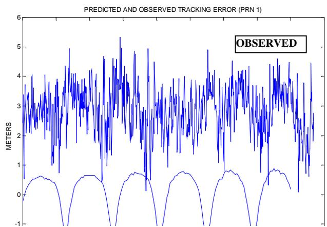
Figure 8: Comparison of predicted and observed code tracking error for a choke ring antenna 6.6 m above the ground (PRN 1).
