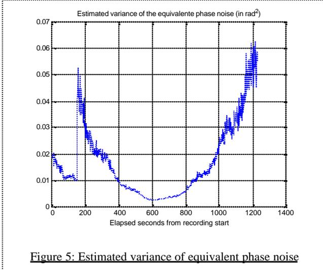
That's the reason why we choose to implement a second order FAB PLL. We know that for second order loops, the bias on the phase measurements is proportional with the LOS acceleration. It means that the noise will be low powered when we need to open the loop bandwidth to track high acceleration and that acceleration will be low when the noise is powerful. This results on a good
