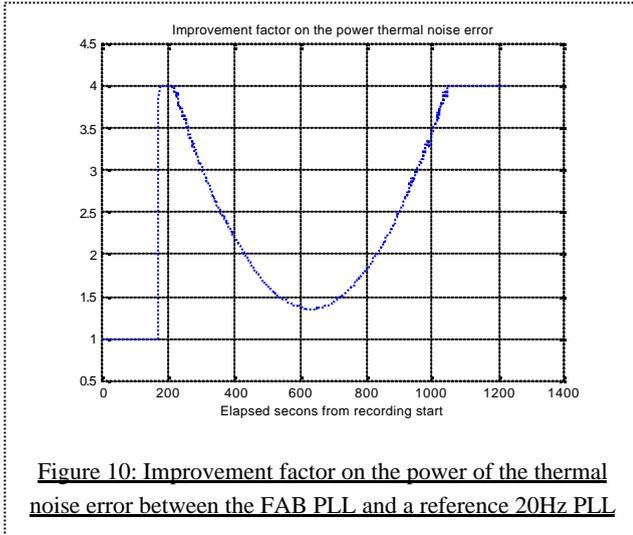
Figure 10: Improvement factor on the power of the thermal noise error between the FAB PLL and a reference 20Hz PLL
