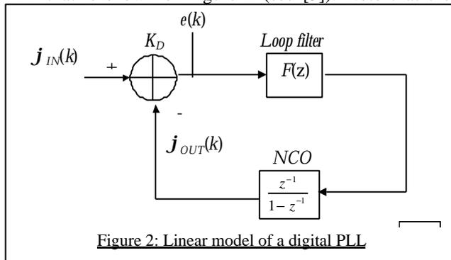
Figure 2: Linear model of a digital PLL
