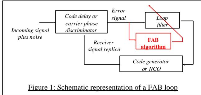
Figure 1: Schematic representation of a FAB loop
