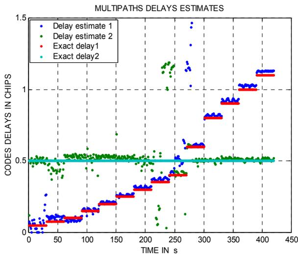
Figures 4.12 Multipath time delay estimation performance with ‘uniform’ distribution for  $\alpha_1=0.1$ ,  $\alpha_2=0.3$  as a function of time in the run (ray 1 delay is constant equal to 0.5 chip, ray 2 delay is as presented above).
