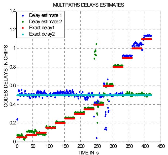
Figures 4.14 Multipath time delay estimation performance with ‘peak intensive’ distribution for  $\alpha_1=0.1$ ,  $\alpha_2=0.3$  as a function of time in the run (ray 1 delay is constant equal to 0.5 chip, ray 2 delay is as presented above).
