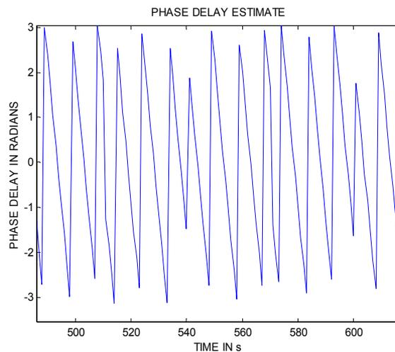
Figure 4.3 Zoom of multipath phase delay estimation performance with 'uniform' receiver configuration for  $\alpha = 0.1$  as a function of time in the run (multipath delay varies by 0.02 chip every 30 s).
