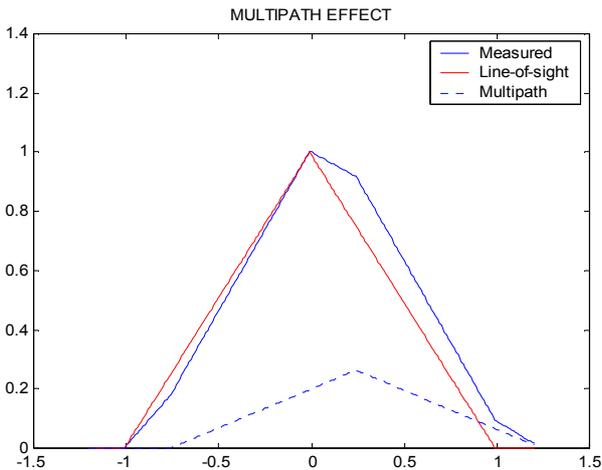
Figure 1.1 Multipath effect on the normalized correlation function.
