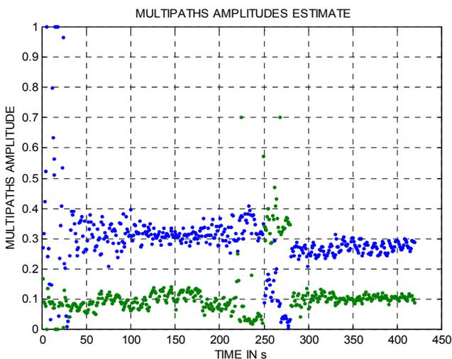
Figures 4.13 Multipath amplitude estimation performance with ‘uniform’ distribution for  $\alpha_1=0.1$ ,  $\alpha_2=0.3$  as a function of time in the run (ray 1 delay is constant equal to 0.5 chip, ray 2 delay is as presented above).
