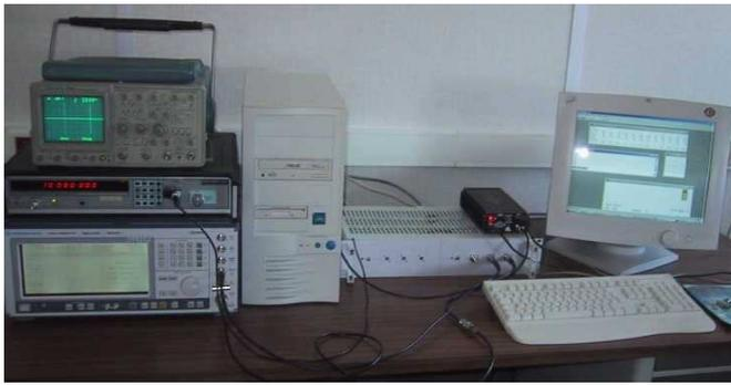
Figure 4: Picture of *evil waveform Test Bed*.
