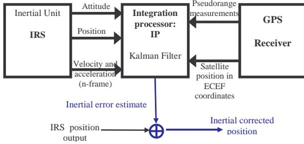
Figure 2. GPS/IRS architecture
