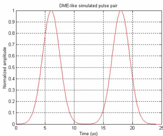
Figure 19 Simulated DME pulse pair
