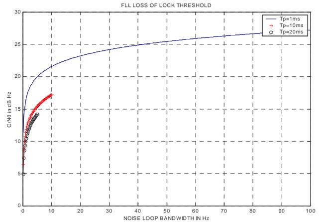
Figure 11: FLL loss of lock threshold on a single data or pilot signal component.
