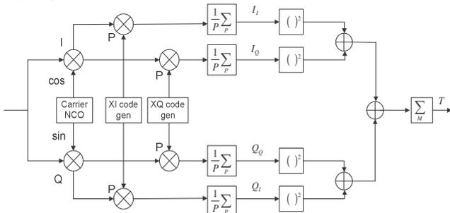
Figure 2: L5 acquisition structure.
