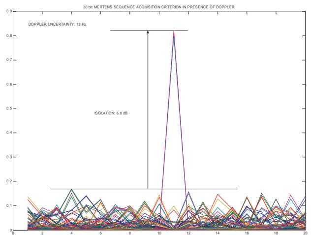
Figure 9: Superposition of the test acquisition criterion (Mertens code) for various Doppler offsets as a function of code lag (residual Doppler=12 Hz).
