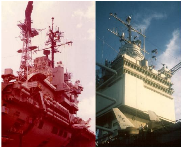
Figure 1. Examples of superstructures where GPS antenna would be mounted Left : USS America (CVA-66) Right : USS Enterprise (CVN-65)
