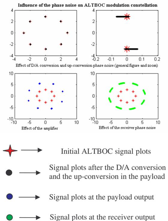
Figure 20: Influence of the payload and receiver phase noise on the ALTBOC modulation constellation
