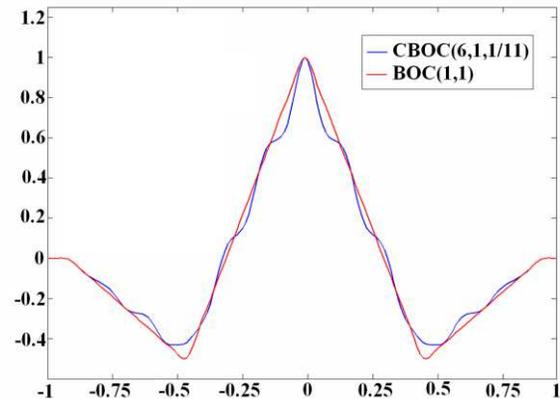
**Figure 4. Normalized Autocorrelation Functions Computed over ±15 MHz Bandwidth**
