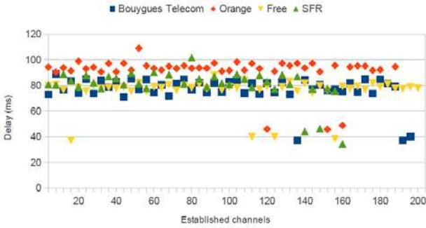
Figure 11. Average delays and jitters for 4 ISPs
