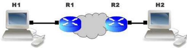
Figure 2. Basic network topology with 2 hosts and 2 routers
