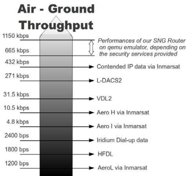
**Figure 15 Air-Ground Data link throughput in year 2012**
