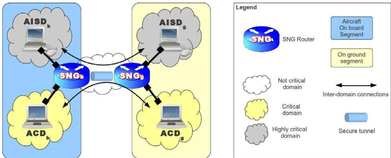
Figure 3 SNG router validation topology
