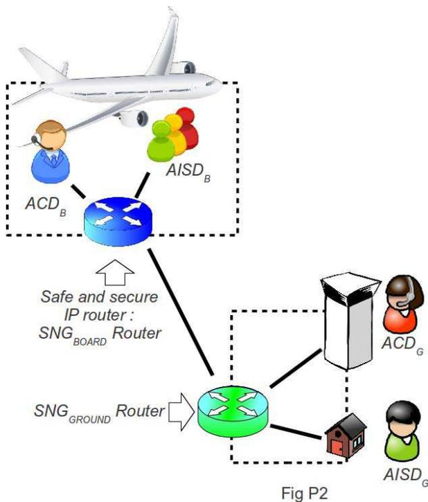
**Figure 8 SNG routers to secure aircraft-ground communications**
