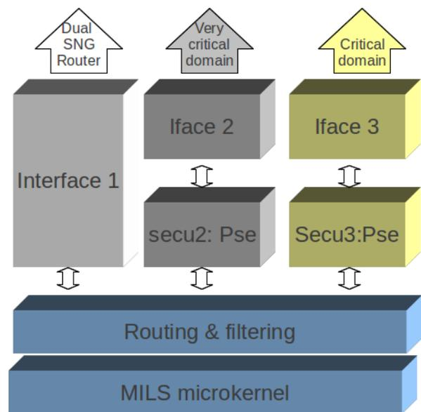
**Figure 5 Example of a possible SNG router configuration**
