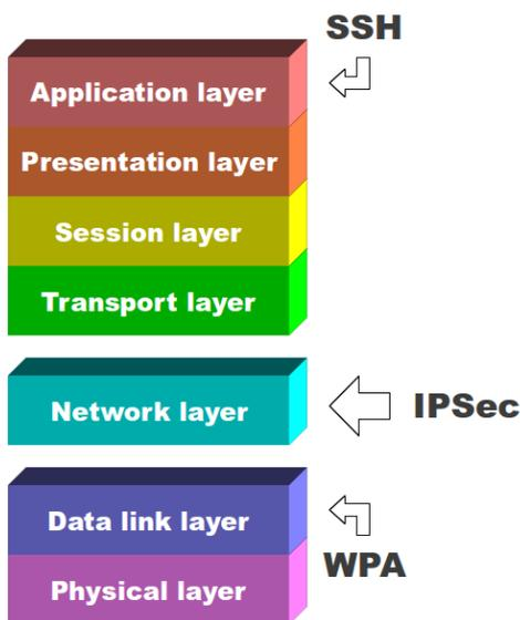
**Figure 1** Some security protocols on the OSI model
