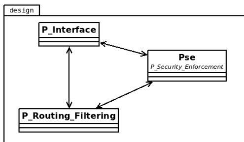
**Figure 4 Simplified design of partitions for SNG routers**
