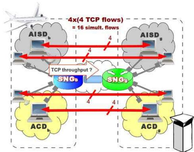
**Figure 13 Measurement of data throughput on multiple paths**
