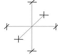
Fig. 3. Antenna constituted by  $N_a = 12$  electric short dipoles .
