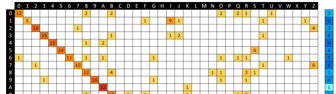
Figure : letter confusion matrix (detail) for the prototype (100cm). Left column shows displayed characters; top row shows subjects' responses. Each intersection of column and row presents the number of occurrence of the stimulus/response pair. The correct responses are displayed on the diagonal of the matrix (stimulus "A" and response "A"...). All other cases are wrong answers, e.g. stimulus "5" and response "S". The far right column (on blue) presents the number of no-responses for each character.
