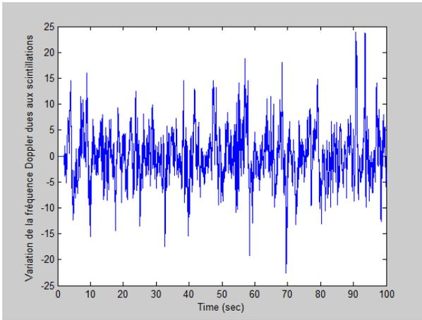
**Figure 5: Variations of the received signal Doppler offset in the intense scintillation case**
