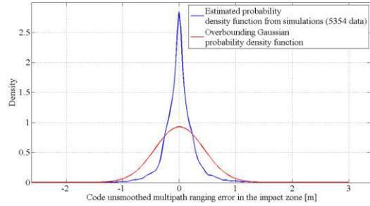
**Figure 7: PDF of the estimated distribution of the code ranging error from simulations in the impact zone of a 10m metallic cube, elevation angle =  $35^\circ$ , azimuth angle =  $0^\circ$ , façade parallel to the Y axis, aircraft speed =  $5m.s^{-1}$  and PDF of the over bounding Gaussian distribution**
