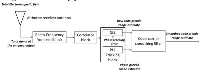
Figure 1: signal processing blocks of a GNSS receiver
