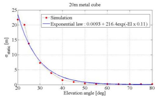
Figure 11:  $\sigma_{static}$  as a function of the elevation angle – impact zone of a 20m metallic cube
