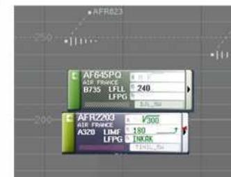
**Layer 3:** The third layer introduces the vertical projection of the aircraft.
