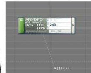
**Layer 4:** The fourth layer connects the projected aircraft position to the electronic strip. This layer enables new working method around the vertical projection.
