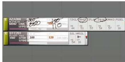
**Layer 1:** The first layer allows the air traffic controller to stick to current working method. The electronic strip has the physical properties of paper: motion, inertia, writable.
