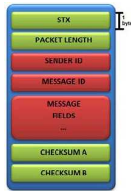
Figure 9: The current standard encapsulation protocol of Paparazzi messages used for RF binary communications
