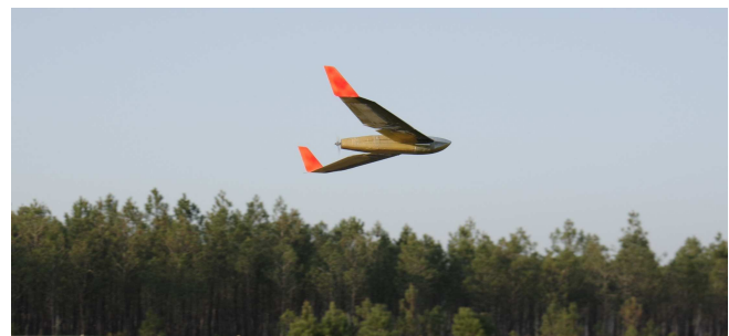
Figure 13: FENIX UAV designed for VOLTIGE project mission requirement
