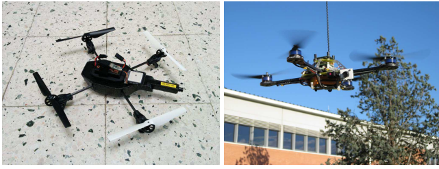
Figure 3: AR.Drone 2 with additional GPS and Asctec Hummingbird frame as two examples of Paparazzi flying rotorcrafts
