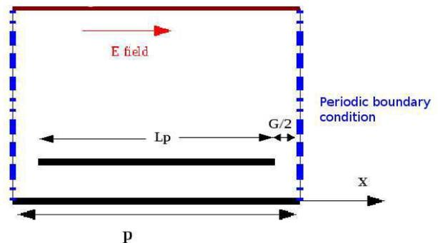
Fig. 1. Configuration of the infinite periodic structure
