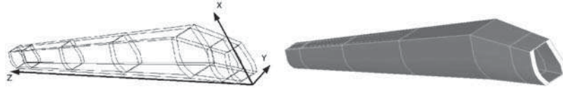
Fig. 7. 3D schema of simplified blade model.
