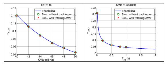
Figure 3 – Comparison of the normalized standard deviation of the CDO without and with a tracking error for different  $C/N_0$  and  $T_{int}$
