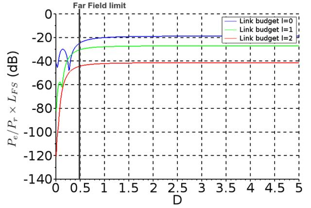
Fig. 8. Test of the  $1/D^{2l+2}$  decreasing assumption.
