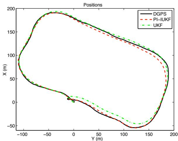
Fig. 2. Experiment: estimated positions UKF vs.  $\pi$ -IUKF
