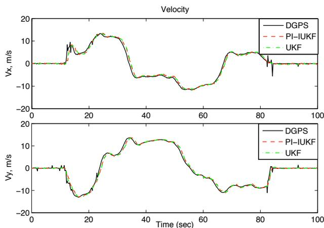
Fig. 3. Experiment: estimated velocities UKF vs.  $\pi$ -IUKF
