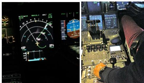
Figure 6: a) the actual A380 full-flight simulator navigation display and its “vertical cut” (white straight line); b) the pilot rotates the button to turn the vertical cut.
