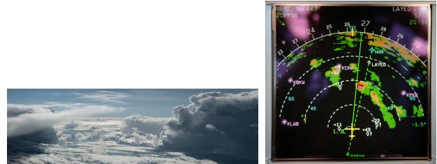
Figure 1: a) a panoramic view looking forward from the flight deck: dark clouds are towering thunderstorms. Thunderstorms are of course more dangerous in bad light conditions, during dark moonless nights; b) the navigation display of an airliner that shows the radar detection of the clouds on the left (red area indicates a definitely to avoid cumulonimbus).
