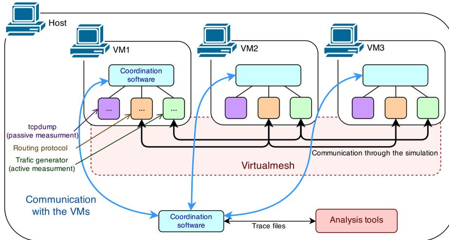
Fig. 1: Testbed implementation
