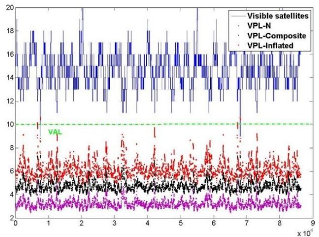
Figure 5- VPLs with  $D_{TH}=5\text{km}$  for GPS + GAL constellations
