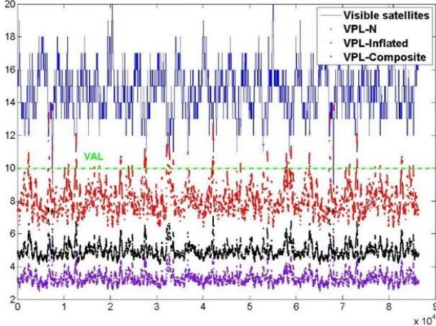
Figure 7 - VPLs with  $D_{TH}=10\text{km}$  for GPS + GAL constellations
