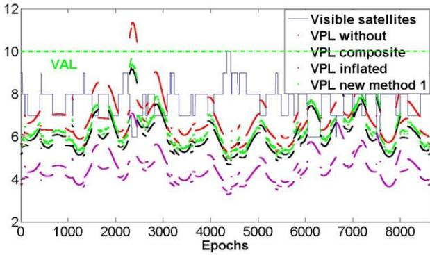
Figure 8 - VPLs with  $D_{TH}=5\text{km}$  for GPS constellation only
