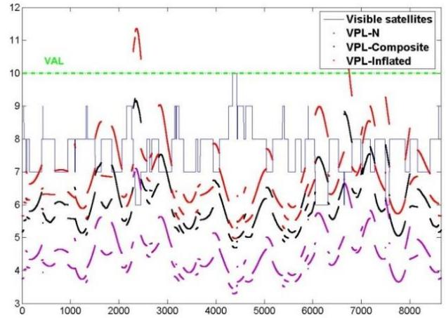
Figure 4 - VPLs with  $D_{TH}=5\text{km}$  for GPS constellation only
