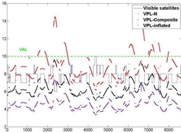
Figure 6 - VPLs with  $D_{TH}=10\text{km}$  for GPS constellation only
