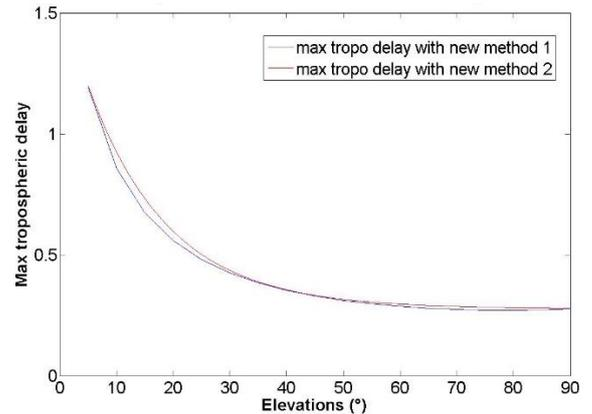
Figure 10 -  $\mu_{max}$  with the 2 new methodologies
