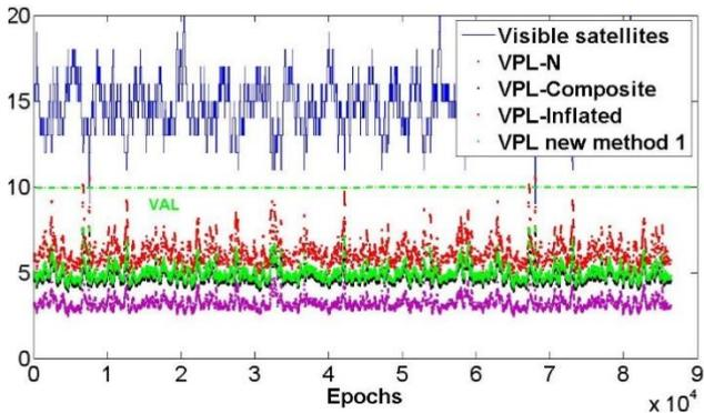
Figure 9-VPLs with  $D_{TH}=5\text{km}$  for GPS + GAL constellations
